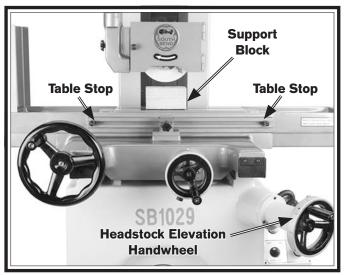
Figure 12. Table and headstock shipping position.
